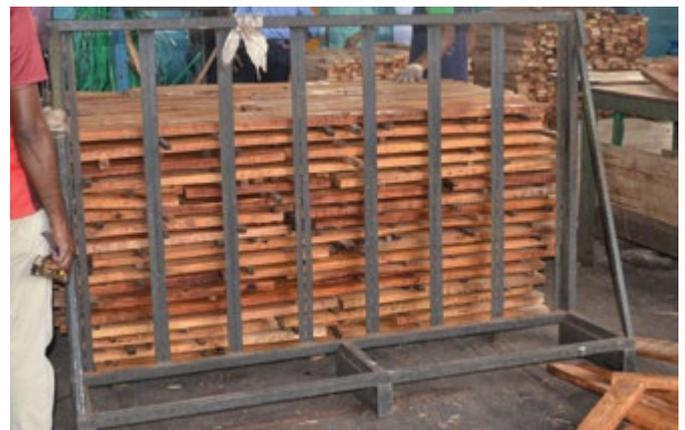
Treated rubberwood is stacked for kiln drying
